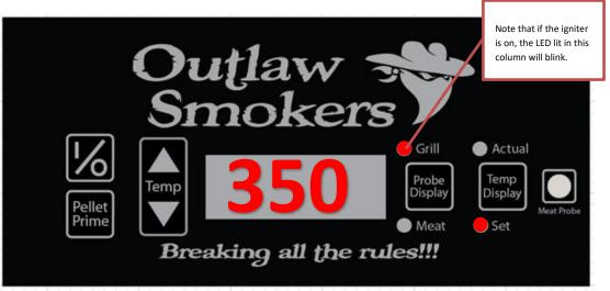
The seven segment display will show the Grill Probe Setpoint temperature by default:
