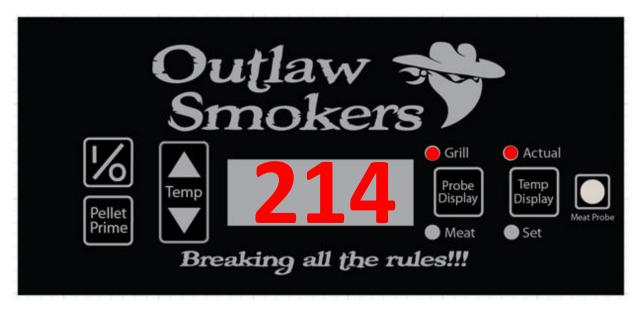
Press the Temp Display button to toggle to the Actual measured temperature of the Grill on the display:
