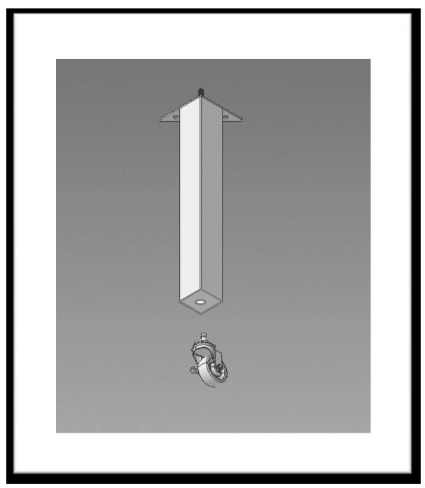
Tools – none Push caster stem in to caster socket. Make sure it is firmly seated. Note: Some grills come with casters already in place.
