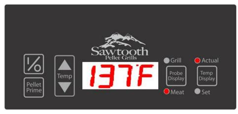
In this state, if the Temp Up or Down buttons are pressed, the display will revert to the Meat Probe Setpoint Display state.
