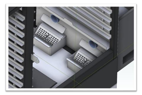
Insert fire tray in to Fire box with "V" down and hole over igniter tube as shown. <u>Igniter tube and</u> igniter should be flush or slightly protrude into the fire tray when installed correctly.
