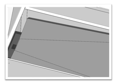
The right drip tray will be installed with the left side resting on top of the left side drip tray and the notched ind resting on the grease tray support rail just above the Fire Shield. The drip tray should rest on the drip tray support.
