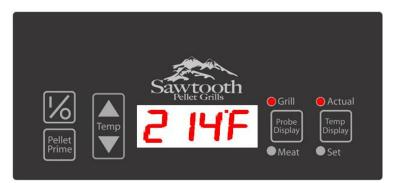
In this state, if the Temp Up or Down buttons are pressed, the display will revert to the Grill Probe Setpoint Display state.
