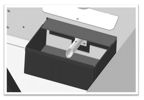
Insert Fire Box into slot in the right side of grill. Fire box should be flush with right side of grill.
