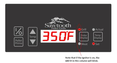
The seven segment display will show the Grill Probe Setpoint temperature by default:
