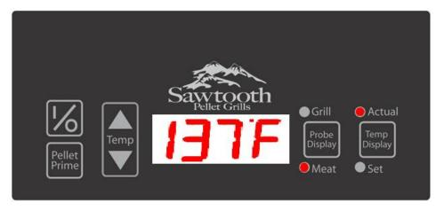
In this state, if the Temp Up or Down buttons are pressed, the display will revert to the Meat Probe Setpoint Display state.
